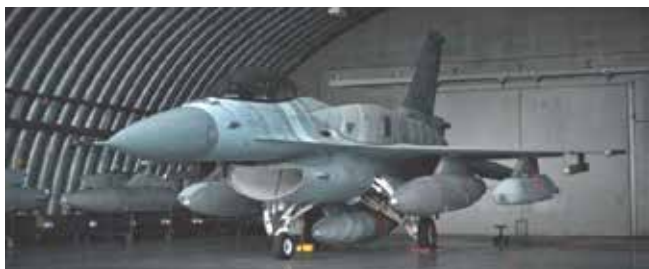
Polish Lockheed Martin F-16 Fighting Falcon fitted with the AGM-158A Joint Air-to-Surface Standoff Missile (JASSM). Source: Polish Ministry
